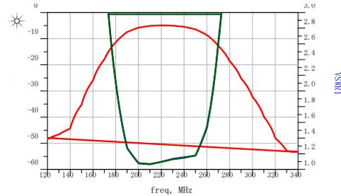
Broadband Insertion Loss VS Frequency ( $T_A=25^\circ\text{C}$ )
