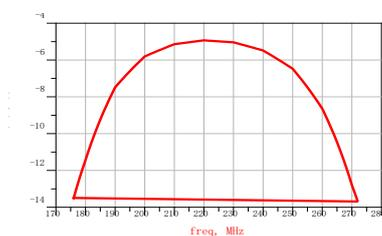
Insertion Loss & Return Loss VS Frequency ( $T_A=25^\circ\text{C}$ )
