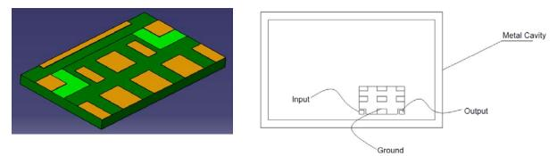
3. This filter should be soldered 2mm (at least) away from mental cavity, in order to avoid degrading filter's performance by mental cavity. Refer to the below figure.
