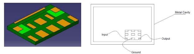
3. This filter should be soldered 2mm (at least) away from mental cavity, in order to avoid degrading filter's performance by mental cavity. Refer to the below figure.
