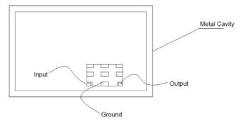
3. This filter should be soldered 2mm (at least) away from mental cavity, in order to avoid degrading filter's performance by mental cavity. Refer to the below figure.
