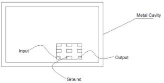
3. This filter should be soldered 2mm (at least) away from mental cavity, in order to avoid degrading filter's performance by mental cavity. Refer to the below figure.
