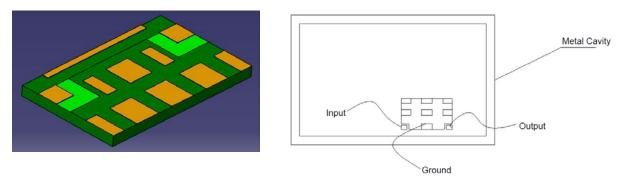
3. This filter should be soldered 2mm (at least) away from mental cavity, in order to avoid degrading filter's performance by mental cavity. Refer to the below figure.
