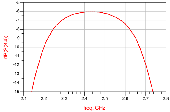
Pass band 4 Insertion Loss VS Frequency ( T_A=25^\circ\text{C} )
