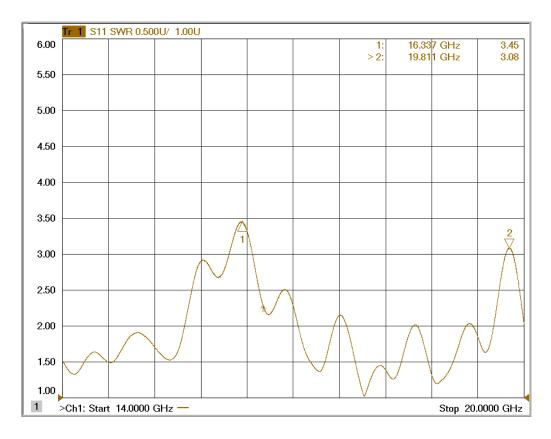
Note: Where accurate measurements are required on a high VSWR signal source, a high quality 10 dB coaxial attenuator, such as a Keysight 8493C, will drastically reduce mismatch uncertainty and provide more accurate measurements.
