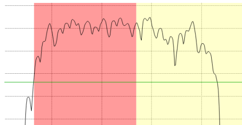
Figure 36: A signal breaking a flat baseline threshold and falling partially within an exclusion zone (the yellow shaded portion). Only the unexcluded part of the signal is considered an event (the red shaded portion).
