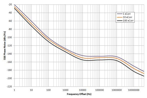
Figure 7: 6GHz Noise Floor Measurements
