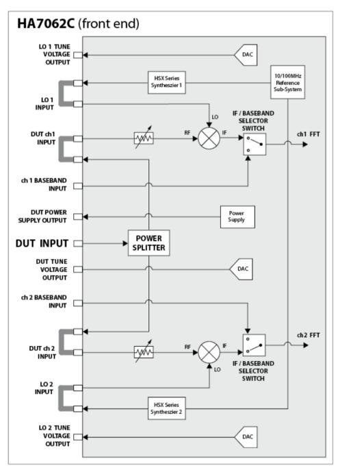
Figure 1: HA7062C Front End Block Diagram
