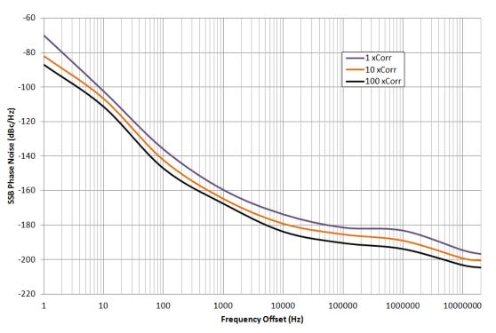
Figure 4: 100MHz Noise Floor Measurements
