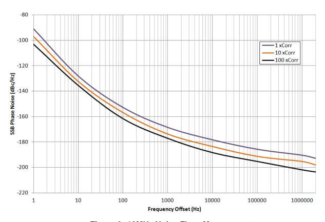
Figure 3: 10MHz Noise Floor Measurements
