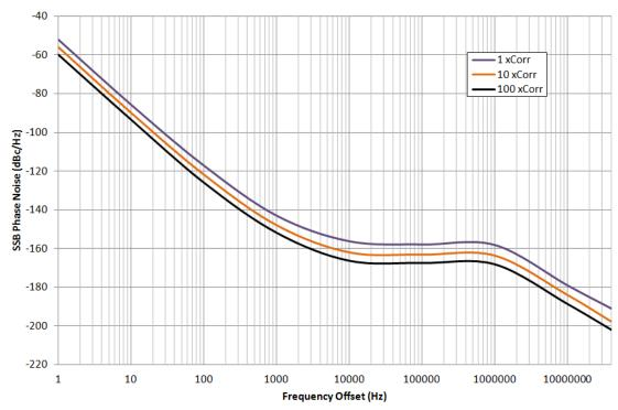
Figure 5: 1GHz Noise Floor Measurements
