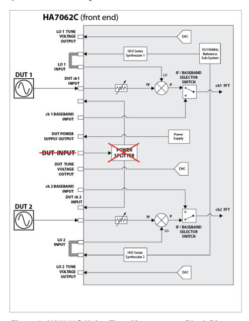
Figure 2: HA7062C Noise Floor Measurement Block Diagram
