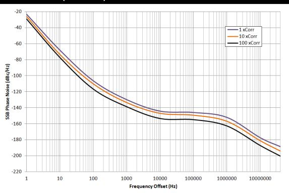
Figure 6: 3GHz Noise Floor Measurements
