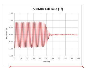
Figure 3b: Pulse Mod Fall Time, fc = 530MHz
