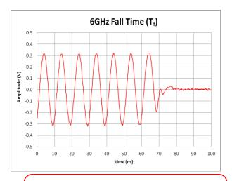
Figure 4b: Pulse Mod Fall Time, f<sub>c</sub> = 6GHz
