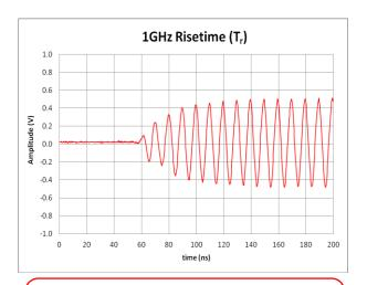
Figure 2a: Pulse Mod Rise Time, fc = 1GHz
