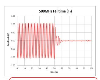
Figure 1b: Pulse Mod Fall Time, fc = 500MHz
