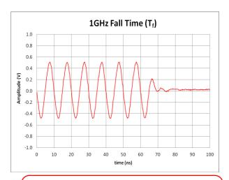
Figure 2b: Pulse Mod Fall Time, fc = 1GHz
