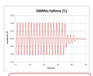
Figure 2b: Pulse Mod Fall Time, f<sub>c</sub> = 500MHz
