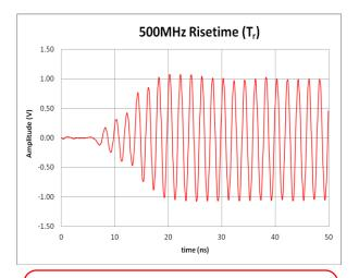
Figure 2a: Pulse Mod Rise Time, fc = 500MHz
