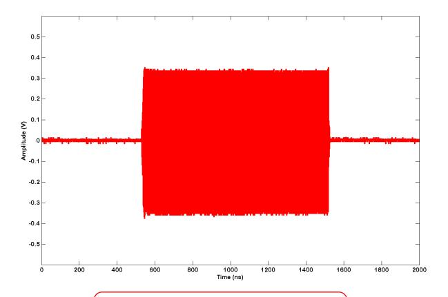
(Figure 1: Self Pulse Mod f<sub>c</sub> = 500MHz, 1us Pulse<sup>2</sup>)
