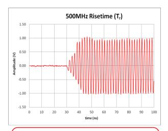
Figure 1a: Pulse Mod Rise Time, fc = 500MHz
