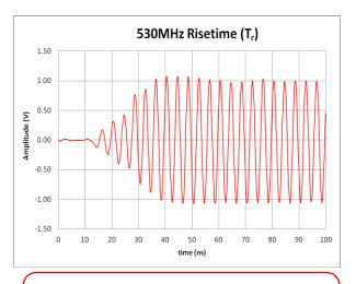
Figure 3a: Pulse Mod Rise Time, fc = 530MHz
