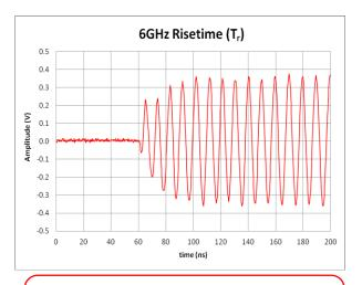
Figure 4a: Pulse Mod Rise Time, fc = 6GHz
