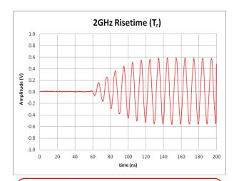
Figure 3a: Pulse Mod Rise Time, fc = 2GHz
