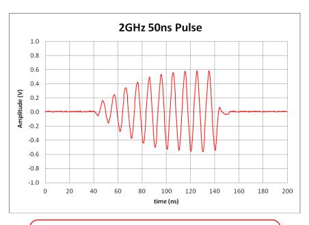
(Figure 5: Self Pulse Mod f<sub>c</sub> = 2GHz, 50ns Pulse<sup>2</sup>)
