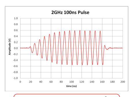
(Figure 6: Self Pulse Mod fc = 2GHz, 100ns Pulse<sup>2</sup>)
