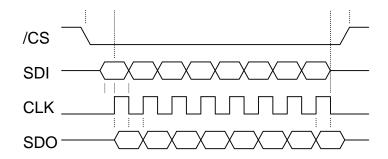
The figure above demonstrates bit level timing where data is sampled into and out of the module on the rising edge of SCLK (Slave Clock). Data out is valid on the falling edge of SCLK.
