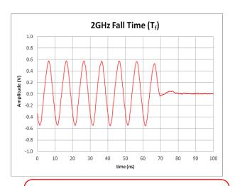
Figure 3b: Pulse Mod Fall Time, fc = 2GHz
