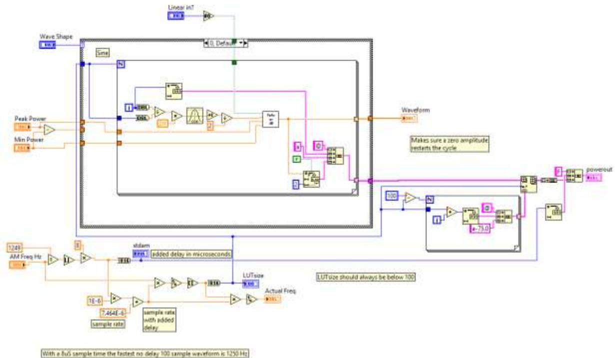
How the delay is calculated in the Windfreak SynthHD GUI:
