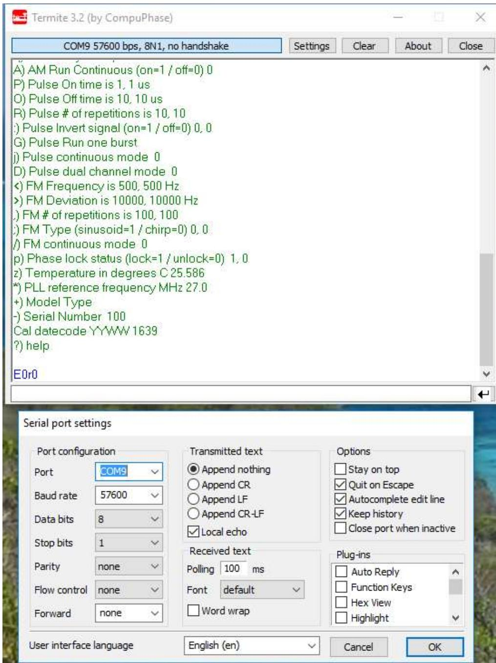
At the bottom of the screen is the command and data entry box. Send a “?” to have the SynthHD respond back with a list of its commands. Try sending a frequency or power command like already mentioned and watch for the change on your spectrum analyzer. Also try sending queries like “f?” to have the SynthHD respond with the status of that particular command. All responses are terminated with a “\n” which is a LF (or New Line) character.
