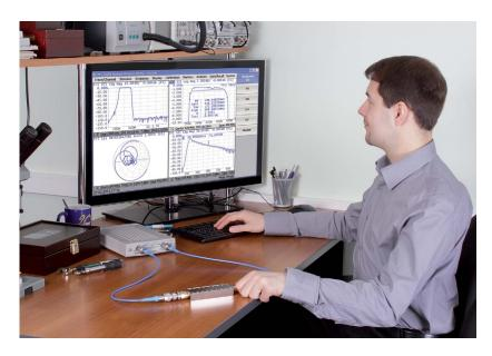
The Planar TR1300/1 VNA is an S-parameter vector network analyzer designed for operation with an external PC. It connects to any Windows-based computer via USB and delivers accurate testing and measurement through a platform that can keep up with constant advancements as well as be remotely accessed.
