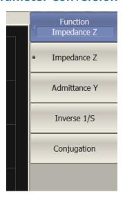
The function allows conversion of the measured S-parameters to the following parameters: reflection impedance and admittance, inverse S-parameters, and conjugation.
