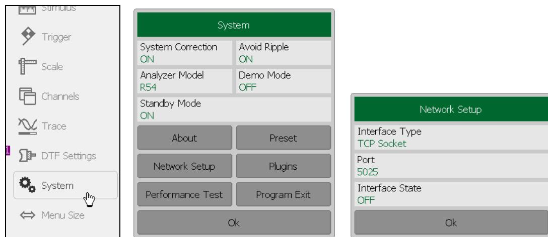
To enable/disable remote control via Socket protocol use the following softkeys:
