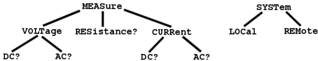
Each tree structure forms a functional system. The base of the tree is called root, e.g. MEASure and SYSTem. Each functional system can have subsystems of lower level. The final nodes are called leaves. The entire sequence from the root to the leaf makes up the command. For example, part of SOURCe functional system looks as follows:
