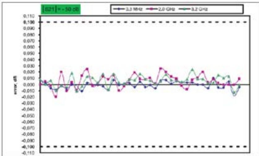
Low trace noise allows for particularly high-precision measurements. This graph shows the variation of the absolute value of the measurement error of  $S_{21}$  and  $S_{12}$  with a value of  $|S_{21}|$  and  $|S_{12}|$  -50 dB, using 42 different instruments. With the model's specified accuracy of  $\pm 0.1$  dB, the trace clearly shows that the variations within the instrument pool is well below that figure. This confirms the precision of the instrument.
