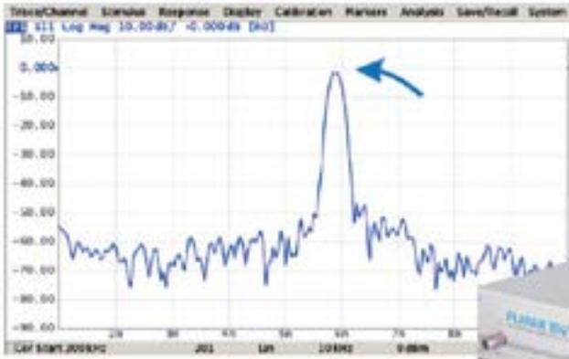
This function performs conversion from frequency domain into response of the DUT to various stimulus types in time domain. Modeled stimulus types are bandpass, lowpass impulse, and lowpass step. The time domain span is arbitrarily between zero to maximum, which is determined by the frequency step. Windows of various shapes are used for tradeoff between resolution and levels of spurious sidelobes.
