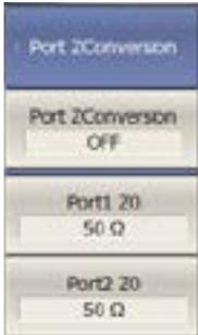
This function converts the S-parameters measured at a 50 Ω port into values which would be seen if measured at a test port with arbitrary impedance.
