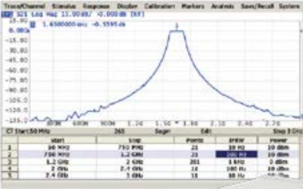
The VNA has a large frequency range with the option of frequency scan segmentation. This allows for optimal use of the instrument to realize maximum dynamic range while maintaining high measurement speed.
