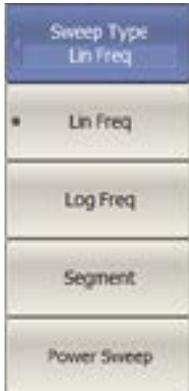
**Sweep type:** Linear frequency sweep and logarithmic frequency sweep are performed with fixed output power. Linear power sweep is a fixed frequency.
