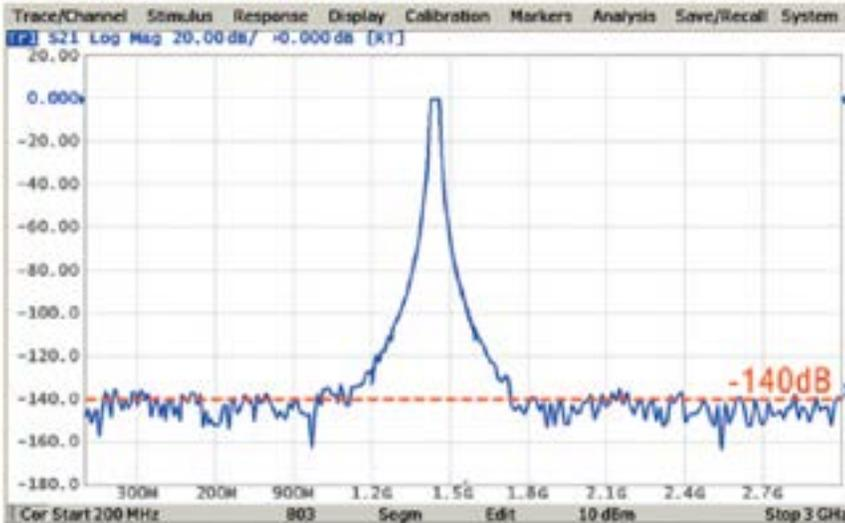
Typical dynamic range of 140 dB, typ. is achieved through the entire frequency range (10 Hz IF BW). Seen here is the maximum dynamic range achieved when using 10 IF BW and an output power level of 10 dBm.
