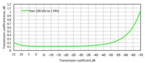
Specifications are based on matched DUT, and IF bandwidth of 1 Hz
