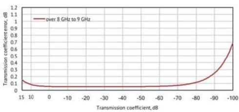
Specifications are based on matched DUT, and IF bandwidth of 1 Hz
